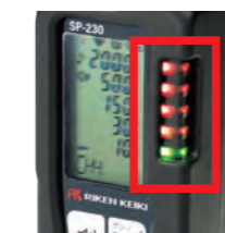
Gas alarm state
