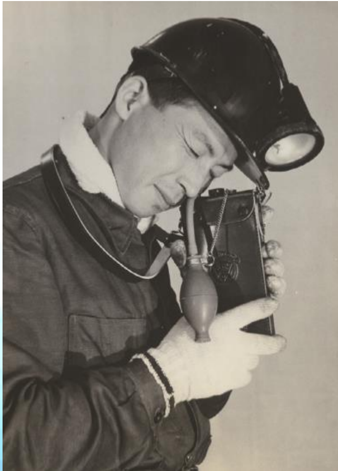
Methane gas measurements in coal mine
